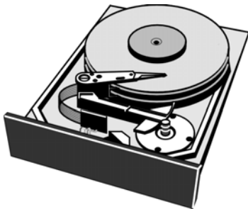
fig. 20: Hard disk, interior
